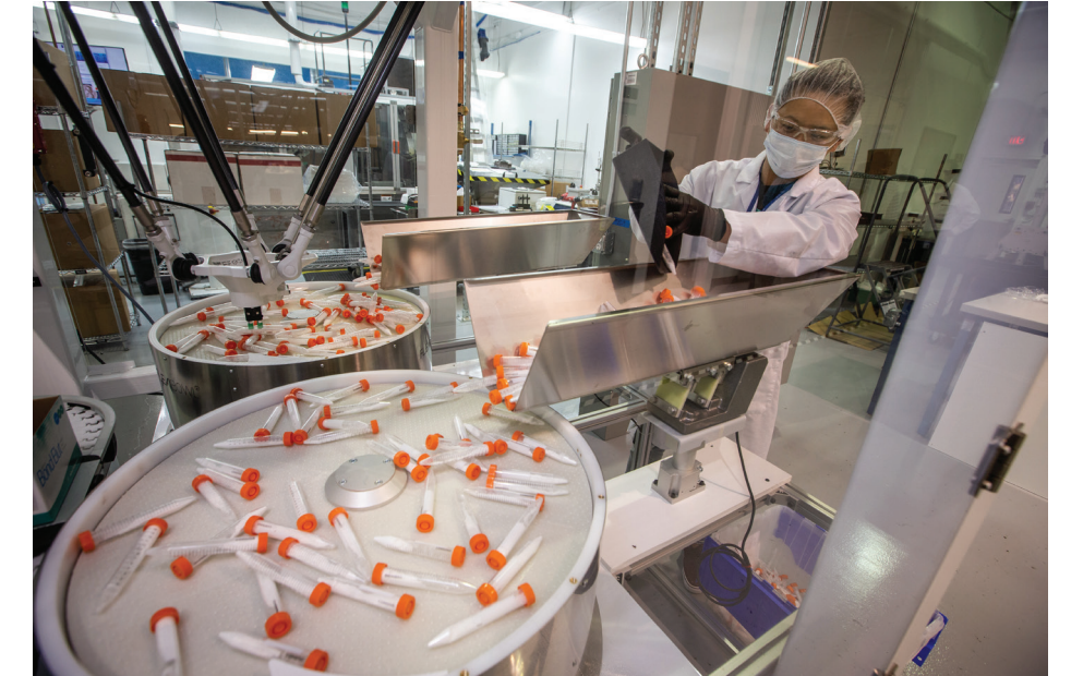
Left, “Rosie the Robot” works in the Sample Prep area, feeding empty tubes onto machines, filling them with media, then capping them. The finished products are sent over to a spider-like robot that quickly and carefully packs them into boxes, ready for customers.
