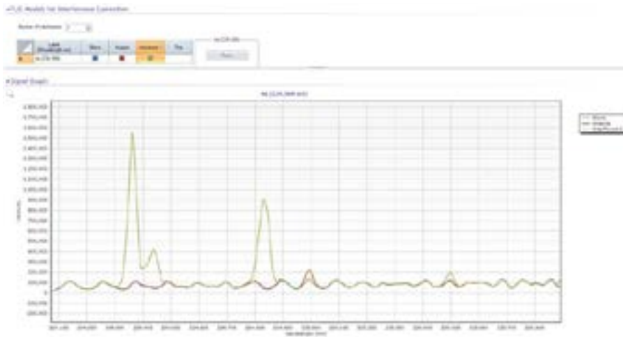
Figure 1. Illustration of spectral interference correction using FLIC. Figure 1 represents the FLIC page showing blank, analyte and interferent spectra
