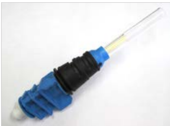
Figure 1. The inert MP-AES torch
