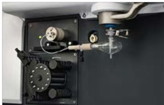
Figure 1. Agilent 4210 MP-AES with Agilent Advanced Valve System (AVS 4) four port switching valve
