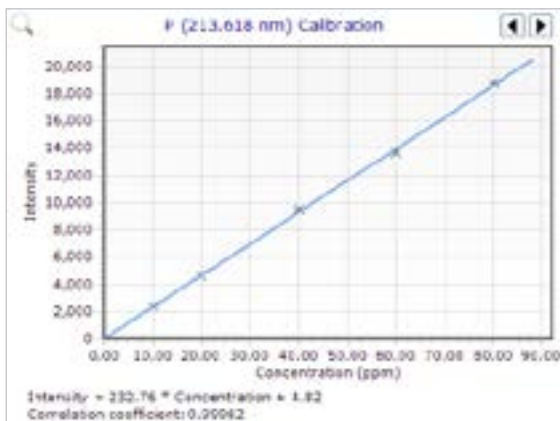
Figure 1. Calibration curve for phosphorus
