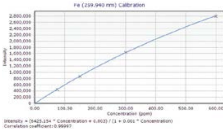
Figure 2. A typical non-linear calibration curve in MP-AES
