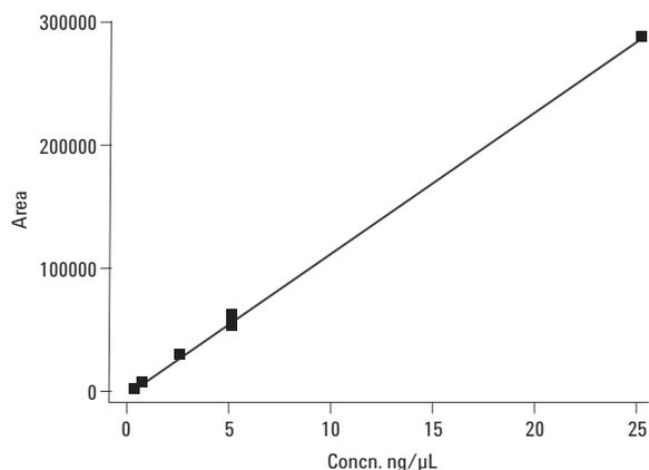
**Figure 4. Codeine linearity. Plot of codeine extracted ion (ms/300.0–300.2) chromatographic peaks measured from 50-pg injected on-column to 25-ng on-column. TOF detector saturated at 50 ng.**
