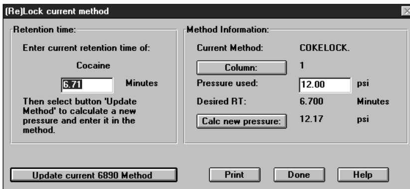
**Figure 3. Column pressure recommendation for retention time locking and method update (as found on the RTL software for the GC ChemStation).**
