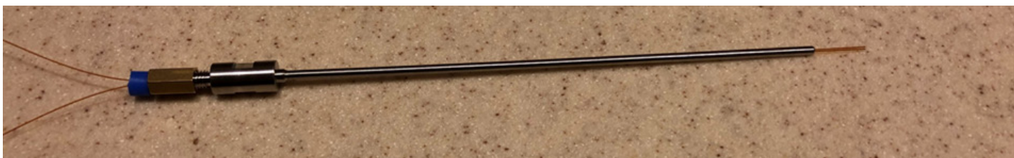
Figure 5. Column placement exaggerated to illustrate the proper use of the column insertion tool.
