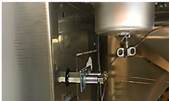
Figure 7. Configuration 2: Inert tee installed on the MS transfer line with the QP and GC analytical columns.
