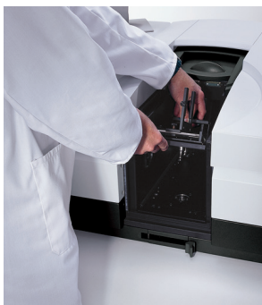
2. Position accessory over mounting holes
