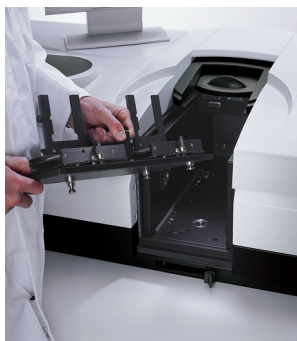
1. Insert accessory into the sample compartment
