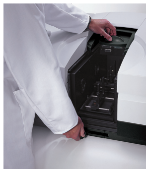
3. Flick the switch to lock the accessory down
