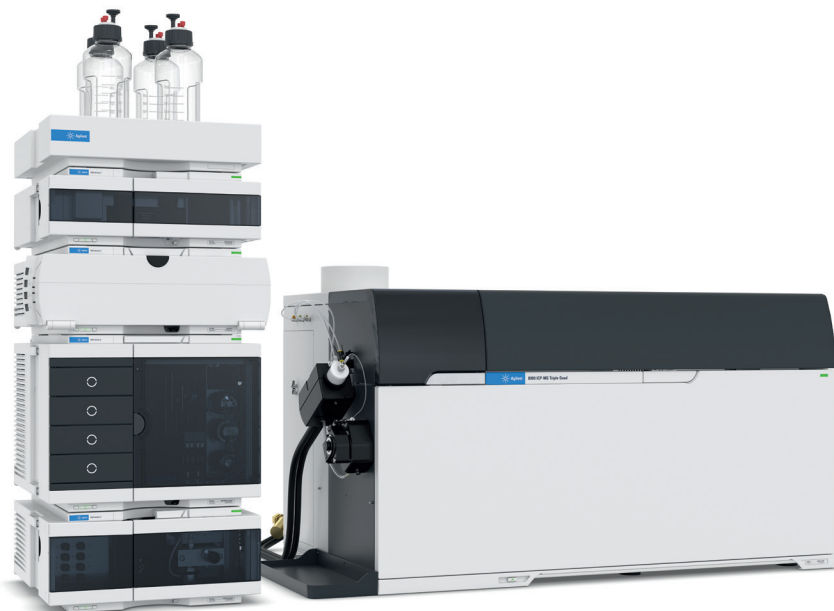
Figure 1. Agilent 8900 ICP-MS coupled to an Agilent 1260 HPLC for speciation analysis and protein mass purity measurements.
