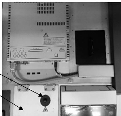
**Figure 14.** Dewar hole on spectrometer
