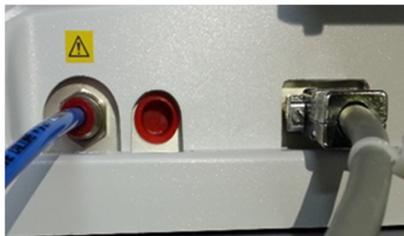
**Figure 9.** Upper rear connectors on the microscope. Left to right: Purge fitting to gas supply; Video out to video capture card installed in the computer (non-ToupCam models only); Microscope to spectrometer EXT DET 1 or EXT DET 2 connection (see Figure 7).
