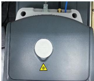
**Figure 15.** Top of the microscope showing the liquid nitrogen plug
