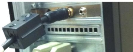
**Figure 10.** Video capture card (installed in PC) with 'Video out' cable connected
