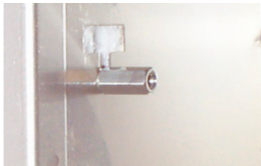
Figure 17 Mounting a standoff in a tee slot
