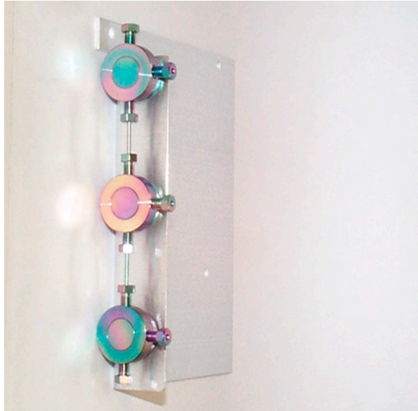
Figure 14 Completed pneumatic coupler assembly
