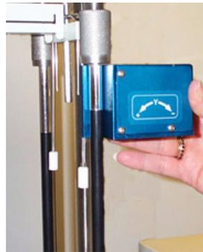
**Figure 14** Electronic Level Sensor Placement
